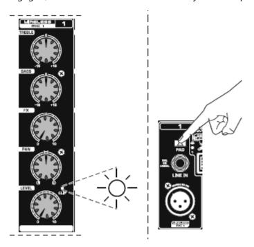
12, Adjust the left-right position of a channel in the stereo field by turning the channel' s PAN knob.
