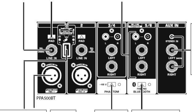
AUX IN inputs route stereo signals directly into the main mix through either a sginle1/8' / TRS stereo plug or left and right
