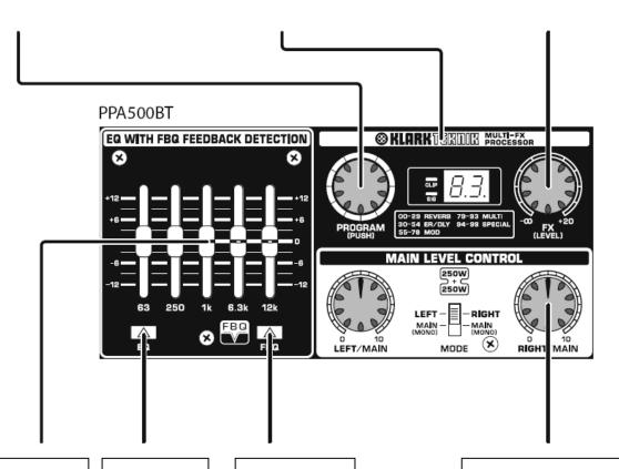
GRAPHIC EQ adjusts specific frequencies in the sound spectrum.
