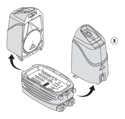
4,Stand the mixer upright.(Make sure the include speaker cables can reach both speakers)
