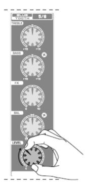
11, If a channel' s CLIP LED lights, press the PAD button. If the PAD button is already engaged, turn the LEVEL knob down. Always use the pad button with line level inputs.
