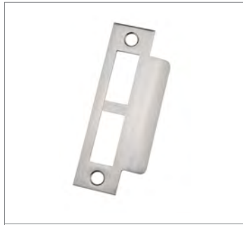
Brass Standard Strike Plate 1 7/8" wide x 4 7/8" high Supplied with Mortise Locks unless door thickness is specified as 2" or greater
