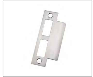
Brass Extended Strike Plate 2 1/2" wide x 4 7/8" high Supplied with Mortise Locks when door thickness is specified as 2" or greater
