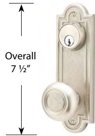
• Belmont Knob with Keyed Belmont Plate • Two standard 2 1/8" door preps • 3 5/8" Center to Center hole spacing
