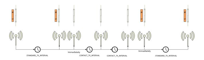
Figure 7 - Magnet contact sensor-controlled reporting interval
