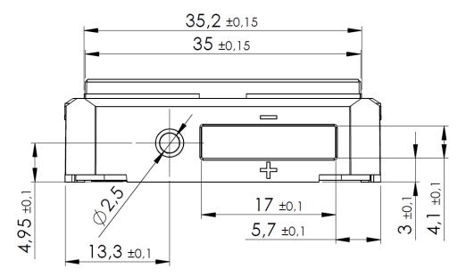
Figure 59 - Front view of STM 550 module
