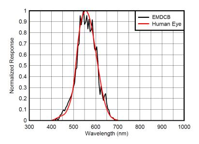
Figure 8 - Spectrum response of the light level sensor
