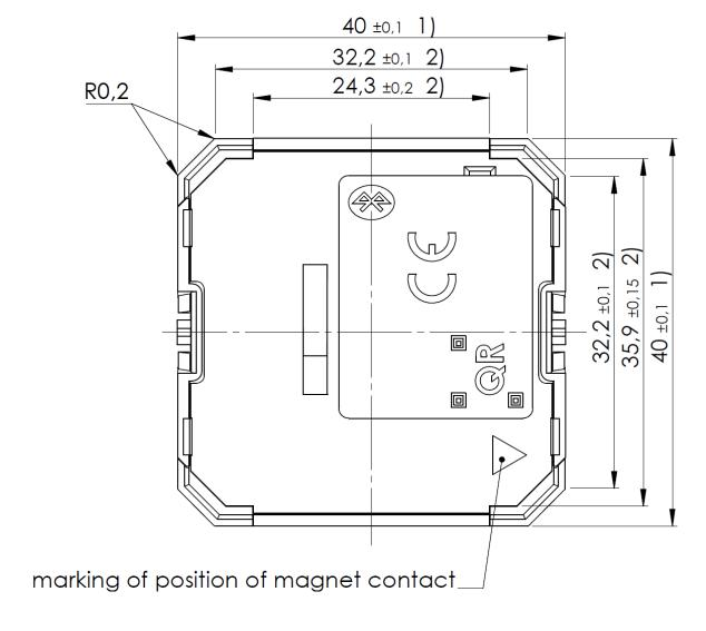
Figure 57 - Bottom view of STM 550 module
