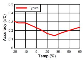
Figure 9 – Temperature sensor accuracy
