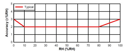
Figure 10 - Humidity sensor accuracy
