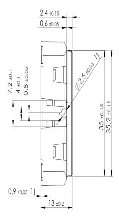
Figure 60 - Side view of STM 550 module
