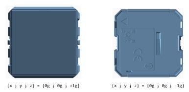
Figure 62 - Acceleration vector based on device orientation
