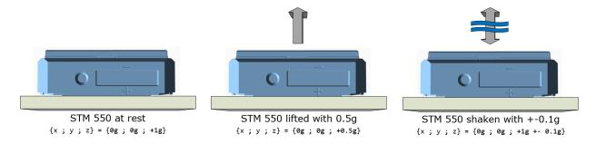
Figure 65 - Acceleration vector changes based on motion or vibration
