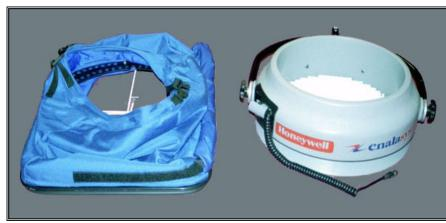
Now the Supply Airflow Hood must be attached to the Supply Power Ring. This is done by fitting the circular end of the hood over the bottom lip of the ring. The correct orientation of the Power Ring is indicated by the logo, which should be upright and readable.
