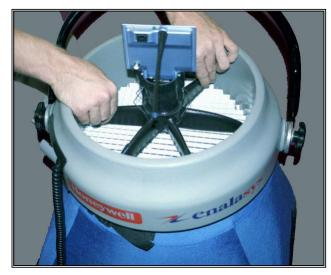
Next, the Supply Sensor Board / Manifold assembly must be attached to the Supply Airflow Hood / Power Ring assembly. Stand the Airflow Hood assembly upright so that the rectangular side is on the floor and the Power Ring is on top. Locate the battery slot on the Power Ring. Lower the Manifold into the Power Ring until it rests on the plastic grid in the center of the Power Ring.
