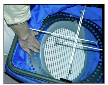
Next the assembly needs to be turned upside down so that the rectangular end of the Airflow Hood is facing up. Locate the four notches on the inside edge of the Power Ring. The hood needs to be twisted while keeping the ring stationary until the four brace rods line up with the notches in the ring (do not insert rods into notches yet). Make sure that the long sides of the hood match with the knobs on the U-shaped yoke.
