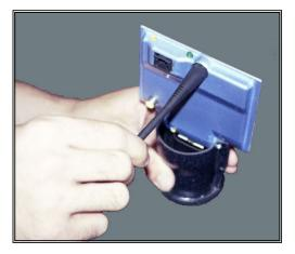
The first step is to attach the antenna to the Supply Sensor board. This is accomplished by first locating the antenna and the antenna mount. The antenna mount is located on top-center of the Supply Sensor board. The antenna is screwed into the mount in a clockwise motion and unscrewed in a counter clockwise motion. Use a firm twisting motion and do not force the antenna, as this may result in damage to the antenna and/or the circuit board.
