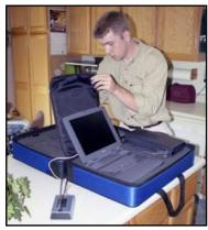
Set up the computer at a convenient location central to the test area. A kitchen table or bar often works well. The eScan-AC components can communicate up to 100 feet, depending on the construction details. Open the case and place the radio receiver as far from the computer as the cord permits, thus reducing potential interference. It is important to place the radio so that the laptop screen will not be directly in the signal path during the test.
