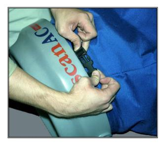
The fabric skirt should fit very snugly around the ring. Now close the two fasteners on the sides of the hood to insure a very tight fit between hood and ring.
