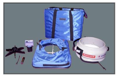
Take an inventory to insure that all parts for the Supply Collector are present and in good repair: Carrying Case, Supply Power Ring, Supply Airflow Hood (residential), Supply Sensor Board, Supply Manifold, Antenna, Battery, and Conversion File Disk.
