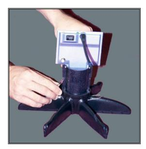
Board cylinder. Apply firm pressure to the clips to get them to seat, but do not force, as this may cause damage to the Manifold and/or Sensor Board. If done correctly, the Sensor Board and Manifold will be firmly attached to one another and will not easily separate.
