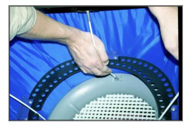
Next, pull the hood's fabric skirt up so that it fully extends. With the skirt fully extended, fit the ends of the four brace rods into the four notches in the Power Ring that they align with. Very firm pressure must be applied to the brace rods to get them to fit in the notches. When properly fitted, the brace rods should bend slightly. This will result in a fully extended Airflow Hood. The fabric should be under tension and stay firmly extended.
