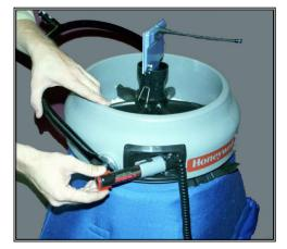
The final part of the physical setup of the Supply DCU is powering up the Sensor Board. First, insert the battery into the Power Ring. The battery will only fit one way into the battery slot. DO NOT force battery, as this can damage the battery and/or the
