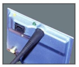
To insure that the Sensor Board is powered and functioning correctly, a "flicker test" must be performed. Press the Transmit Button (the yellow stud on the top edge of the Sensor Board). This should cause the Transmit LED to flicker in response. (The Transmit LED is a green LED on the top edge of the Sensor Board.) A dead battery or malfunctioning circuit board are the most likely causes of a flicker test failure.
