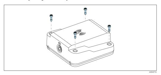
Release the 4 screws, replace the battery, tighten the screws with 1.2 Nm (0.89 lbf ft).
