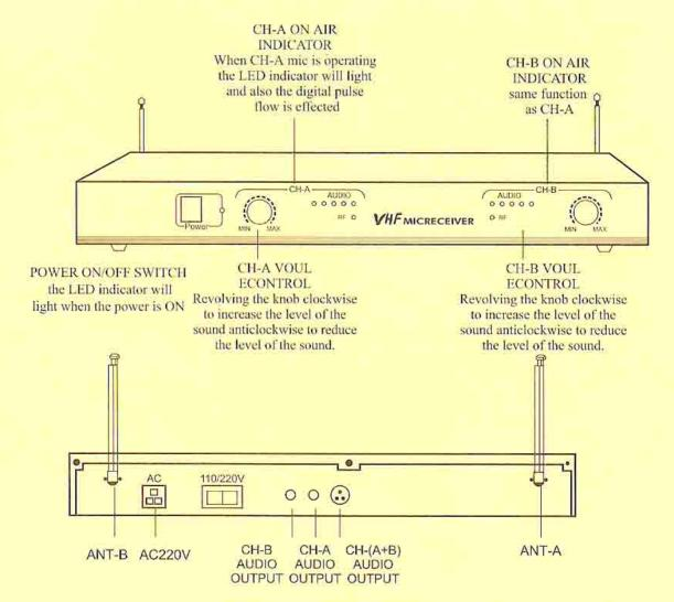
\*Push the power switch to first step, the LED indicator will flash to indicate the carrier frequency is sending out. Push the power switch to second step, the microphone is operating.
