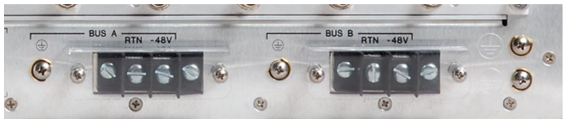
Figure 5-1. Base Station Power Connections (Chassis Rear View)
