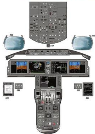
Instrument panel, side panels, overhead panel and pedestal
