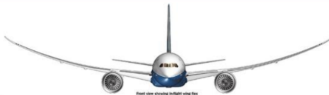
Front view showing in-flight wing flex
