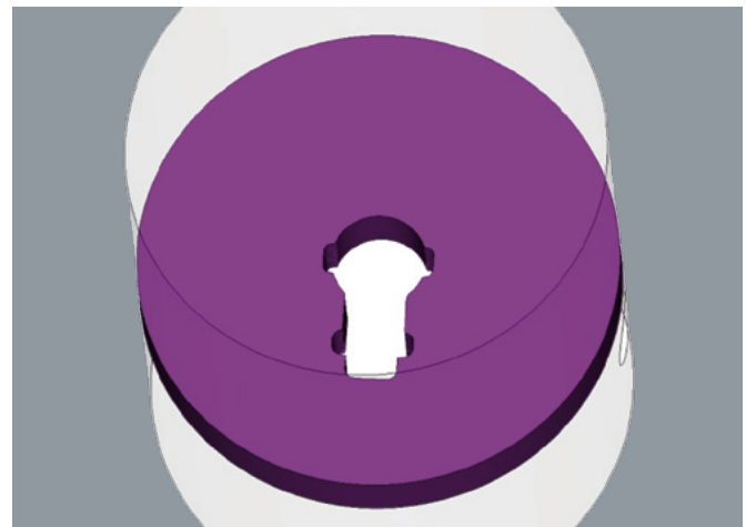
An initial design space for a winch gear support plate optimization exercise. Designs that stay with such a flat, circular shape can be susceptible to warping under the high stresses of competitive sailing.
