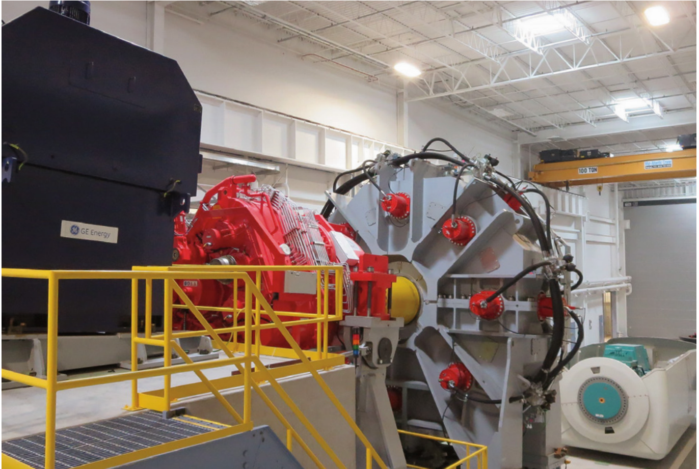
Figure 1. Clemson University's 7.5 MW test bay showing left to right the drive motor, gearbox, load application unit, and nacelle.
