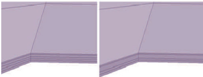
Figure 3: Zoomed views of the finite element mesh before editing (left) and after layers 2 and 3 from the top are merged (right).
