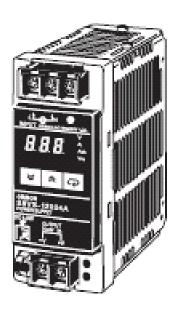
The system power supply is a +24VDC 120W supply capable of providing the source for the base transmitter unit. This supply is a high efficiency switching supply with LED indication of Voltage and current for ease of maintenance. The supply is DIN rail mounted and has covers protecting the AC Mains input and DC output.
