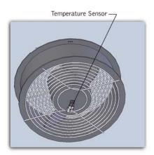
The temperature sensors used in the base transmitter unit are precision semi-conductor temperature to Voltage converters. Additional circuitry is provided to compensate for cable length and to eliminate pulse noise. Both temperature sensors are fed to the DDC module and the information is used both for BITE data and for transmitter monitoring .
