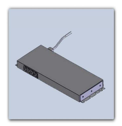
The power distribution module accepts the incoming Mains AC from the transmitter IO panel, and provides a convenient central point of distribution. The module also contains filtering circuitry to reduce EMI. This module accepts standard IEC-C13 and C19 plugs. Each of the various modules within the base transmitter plug into this distribution unit
