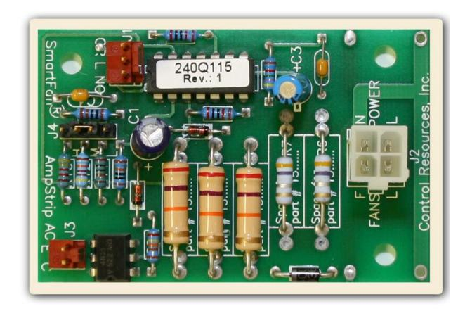
Pictured above is the Alarm current sensor and alarm circuit board mounted on the Magnetron Blower Assembly. This module monitors the Magnetron blower for proper operation via current flow. If the current drops below a pre-set limit due to either motor failure or other faults, the alarm circuit initiates a controlled shutdown of the transmitter thus preventing damage of critical components. There are no adjustments or other periodic maintenance required.
