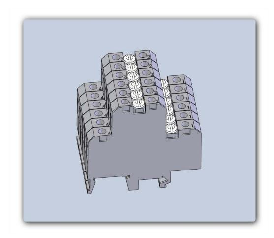
This DIN rail distribution buss is comprised of 6 individual modules connected by a common buss. This distributes both +24VDC and Ground. The terminals are recessed to minimize the risk of short circuit due to foreign debris. All the contacts are properly coated to reduce the risk of corrosion, and to operate without vibration, which could cause individual contacts to loosen. The unit is an industry standard method for proper distribution of low Voltages. No periodic maintenance is required.
