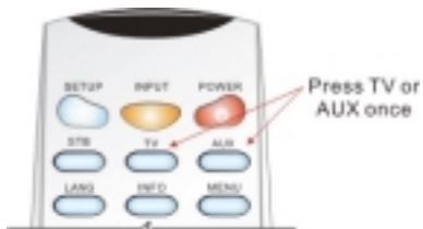
Figure 4-2 Select the device mode
