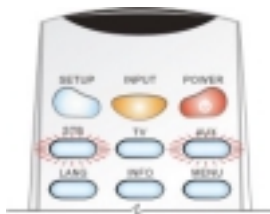
Figure 2-8 URC PLUS in Remote Registration Mode – Step 3 (for box with URC PLUS logo)
