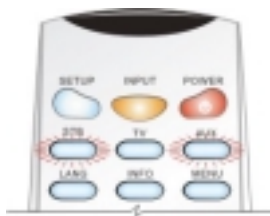
Figure 3-3 URC PLUS in Remote Registration Mode – Step 3 (for Amulet using IR mode)
