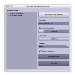
Connect the PRO Mk2 to your computer, and click the top button to establish a connection. The "Show name" and other fields will display any standalone show currently loaded in that box.
