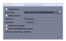
Double-click on a line to open the "Connection Properties" dialog, from where you can configure the connection – which universe(s) to transmit, the network settings (for Art-Net connections) or the hardware serial number (for USB devices).
