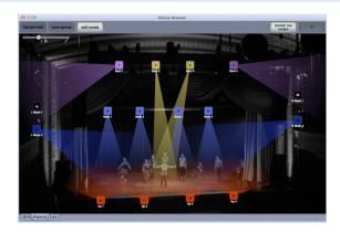
The physical tab is a virtual representation of your rig. Each device appears as an icon against a customisable background image (which can be a picture of your venue, or a simple CAD sketch of the rigging). Each icon can throw a customisable "virtual beam" of light as a simple visualisation tool. The colour & brightness of the icons and virtual beams reflect the actual DMX values being transmitted to the hardware.
