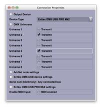
Note that when this option is enabled, you can only transmit ONE DMX universe of data from the PRO Mk2.
