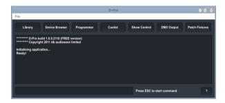
The command line is used for entering text commands - you can view the full command line reference by clicking on the "?" button.
