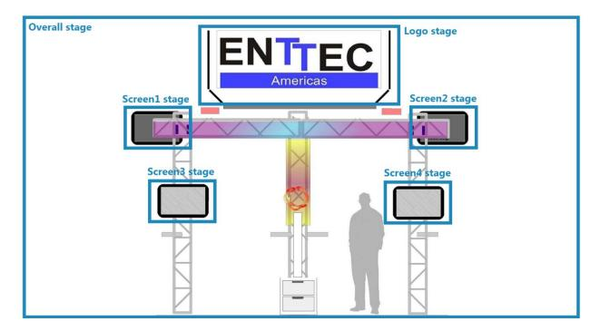
To represent your LED strips and DMX fixtures inside a stage, ELM has a powerful vector-based editor. This way, you can easily draw many types of shapes, including matrices, loops and curves. ELM computes the position of each LED based on your drawing.
