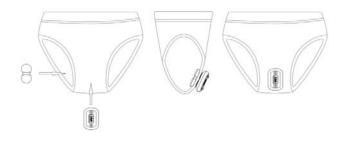
2. The Sensor is attached to special DryBuddy wired briefs using the snaps on one side of the Sensor. These wired briefs are used in place of standard briefs.
