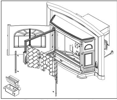
Figure 5: Firebox Components Removal.
