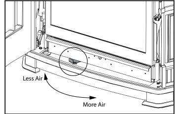
Figure 1: Slider / damper positions.
