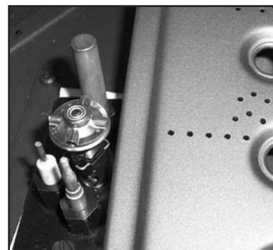
Figure 15: Burner to pilot hood relationship.
