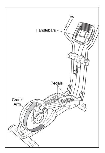
To dismount the elliptical exerciser, wait until the pedals come to a complete stop. **Note: The elliptical exerciser does not have a free wheel; the pedals will continue to move until the flywheel stops.** When the pedals are stationary, step off the highest pedal first. Then, step off the lower pedal.
