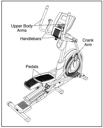
To dismount the elliptical, wait until the pedals come to a complete stop. Note: The elliptical does not have a free wheel; the pedals will continue to move until the flywheel stops. When the pedals are stationary, step off the higher pedal first. Then, step off the lower pedal.
