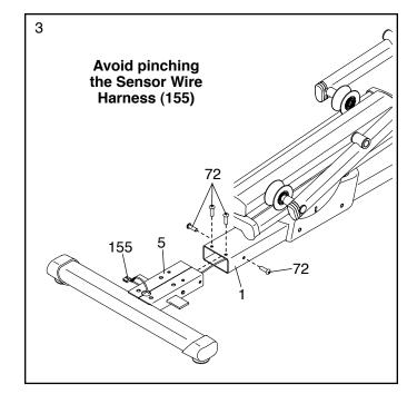
4. Untie and discard the wire tie (not shown) on the Sensor Wire Harness (155).
