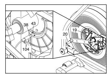
Loosen, but do not remove, the two M4 x 16mm Screws (104). Slide the Reed Switch (38) slightly closer to or away from the Magnet (43). Then, retighten the Screws. Plug in the power cord and press the power switch to the reset position. Turn the left Crank Arm (20) for a moment.
