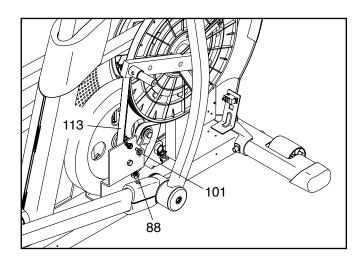
Reattach the right front shield, the shield cover, and the right roller arm.
