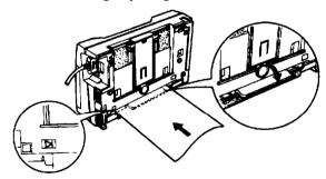
Be sure to raise the flap when not using manual insertion.
