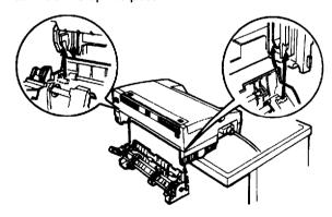
4. Raise the paper-release lever to the continuous-paper position.
