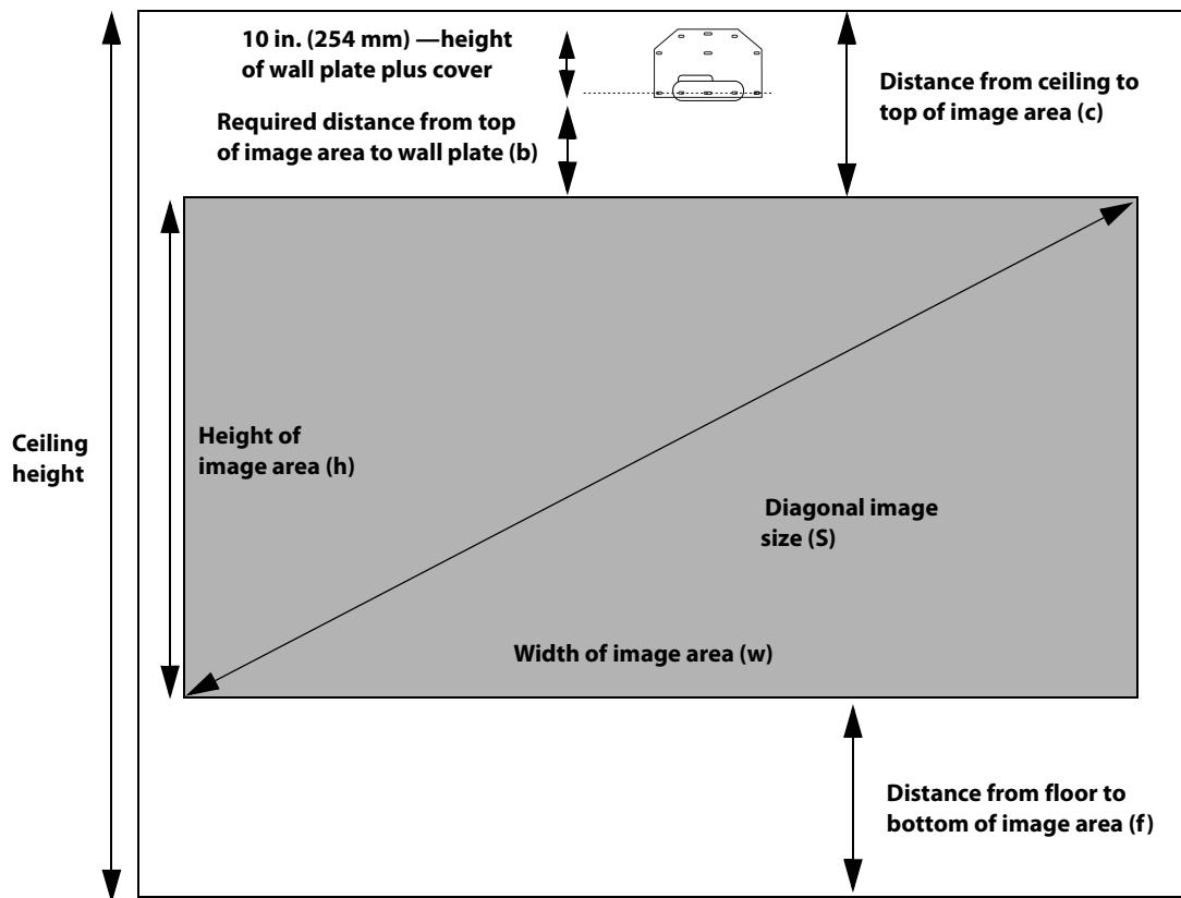
(8) After confirming your image size, use tape or a pencil to mark the distance (b) from the top of the image area on the board to the bottom of the wall plate.
