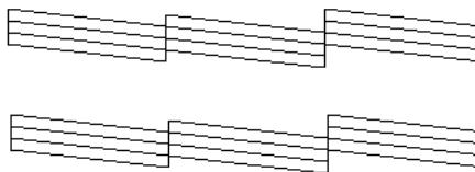
Each staggered horizontal and straight vertical line should be complete, with no gaps in the dot pattern.
