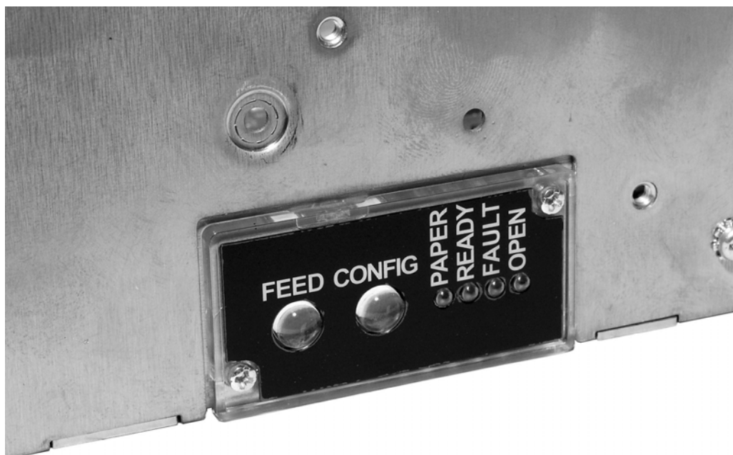
Figure 4. Control panel with FEED and Diagnostics/CONFIG buttons and indicator lights.
