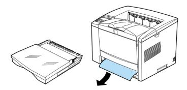
3. Tap the edge of the paper stack. Then reinsert it into the paper tray making sure the paper is evenly aligned and rests below the maximum paper mark.
