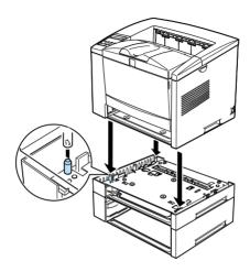
7. Secure the printer to the cassette unit with the screws that come with the cassette unit. Install three of the screws at the location noted below.
