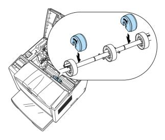
8. Move the paper rollers on the left and right inside and then fit the pins located at the top of the shaft into the paper rollers' grooves.
