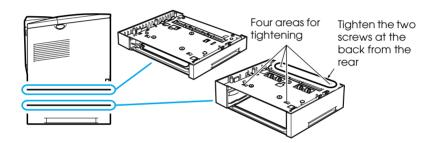
6. Lift up the printer. Make sure the printer and cassette units are facing in the same direction. Aligning the pin on the cassette unit with the hole on the bottom of the printer, lower the printer until it rests securely on the cassette unit.
