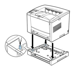
6. Secure the printer to the cassette unit with the screws that come with the cassette unit. Install three of the screws at the locations noted below.
