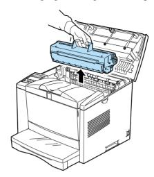
4. Grip the protruding area and move it outside of the two guides located on the left and right.
