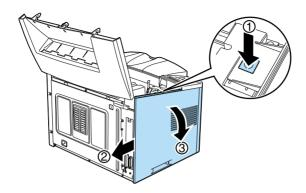
7. Loosen the retaining screws securing the shield cover; then remove the shield cover.
