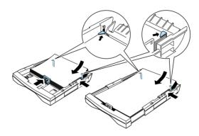
For A4, A5, B5, LT or paper, orient the paper with the long side of paper towards the printer.
