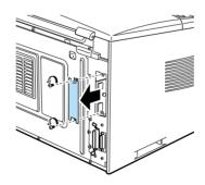
5. With the component side of the optional interface card facing the outside of the printer, slide the interface card into the grooves in the interface slot as shown below. Push it in firmly to lock the card into place.
