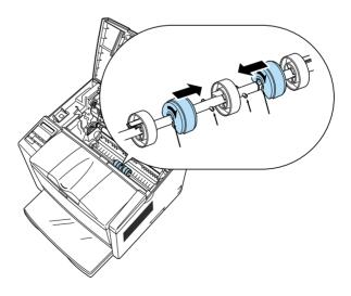
9. Move the left and right guides inside and fix the two left and right paper rollers in position.
