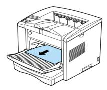
2. Open the printer cover. Be sure to remove any pieces of paper that may have torn off or are remaining in the printer.
