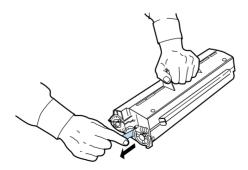
6. Peel off the tape and remove the protective sheet.
