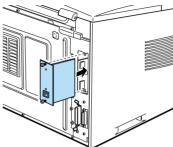
6. Secure the interface card with the two retaining screws.
