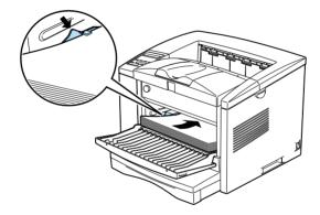
For A4, A5, B5, LT, HLT, EXE, GLT or paper, orient the paper horizontally. The paper tray can close after the paper is set inside it.
