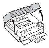
4. Squeeze the tab on the cartridge and lift it up. Dispose of it carefully. Do not take the used cartridge apart or try to refill it.
