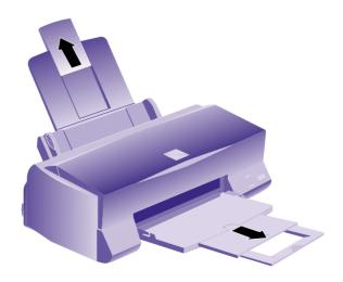
To print on transparencies, remove the paper support and reinstall it in the rear paper support slot.
