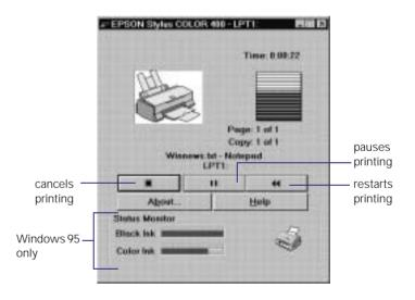
If you're using Windows 95, the Status Monitor box appears inside the Despooler dialog box (as shown above) each time you send a print job. It includes a gauge representing the amount of ink left in the cartridges and an icon that reports the current status of your printer. The icon also alerts you to any printer error conditions.
