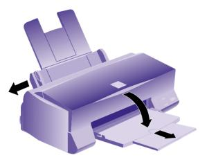
To load long paper, pull out the paper support extension and both output tray extensions.
