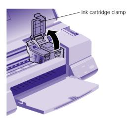
5. Lift the cartridge out of the printer and dispose of it carefully.
