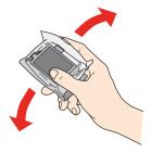
7. Remove the cartridge from the package, but be careful not to touch the green chip on the cartridge.
