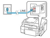
**Note:** If you're connecting to a DSL phone line, you must use a DSL filter or you won't be able to fax. Contact your DSL provider for the necessary filter.
