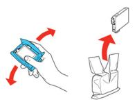
**Caution:** Do not shake the cartridges after opening the packages, or ink may leak.
