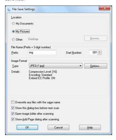
The File Save Settings window may appear after you click **Scan** on the EPSON Scan window. You may also be able to access the window by clicking the electron in the EPSON Scan window.
