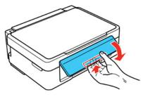
**Caution:** Do not lower the control panel without first squeezing the release bar or you may damage your product.
