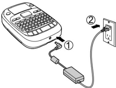
**Caution:** Make sure you use only the AC adapter designed for your LabelWorks printer (C52CB73020) or damage may occur.
