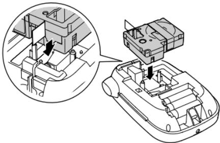
4. If there is excess label, feed the end through the tape guide slot.
