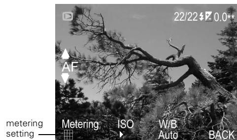
4 Press the bottom left button (next to **Metering**) to change the setting to spot
