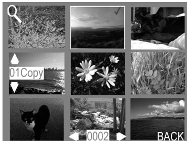
7 Press the **ISO** and **W.B.** buttons (under the left and right arrows) to select photos. A white frame indicates your selection, and the number at the bottom of the screen shows the picture number.
