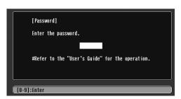
Hold down the Num button on the remote control as you use the numeric keypad to enter the password. Once you enter the password correctly, the screen closes, and projection begins.
