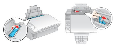
4 Load paper against the right edge and behind the tab, with the printable side face up.
