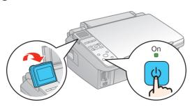
Note: You can raise the LCD display screen for better viewing, if necessary.
