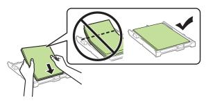
**Note:** Make sure the paper is loaded against the front edge guide and not sticking out from the end of the cassette.
