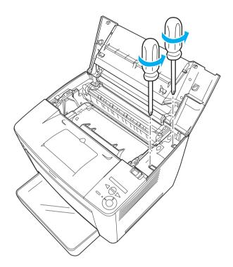
5. Remove the two screws located near the bottom-right edge of the printer.
