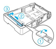
6. Insert the paper size detector at the location of the desired paper size. Push the paper size detector to the left, and then push down the gray stopper to secure the detector, as shown below.
