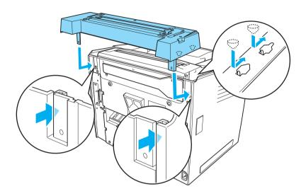
7. Secure the base unit with two screws at the back of the printer by using the wrench that comes with the unit, as shown below.
