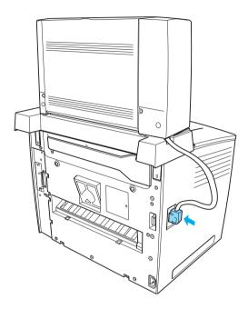
11. Attach four output trays to the main unit by inserting the pins on both sides of the trays into the grooves on the main unit.
