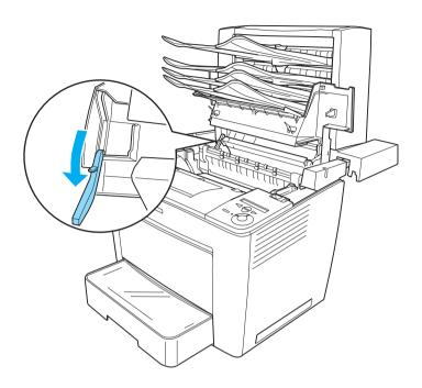
4. Remove the used imaging cartridge, and install a new cartridge by following the instructions described in "Replacing the Imaging Cartridge" on page 257.
