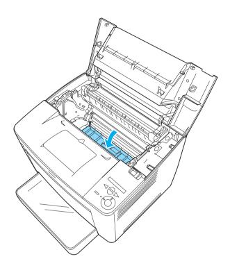
9. Carefully insert the imaging cartridge into the printer, making sure that the pins on both sides of the cartridge are aligned with the grooves inside the printer.
