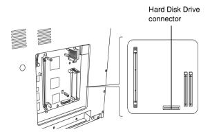
8. Connect one end of the cable that comes with the Hard Disk Drive to the connector on the Hard Disk Drive.
