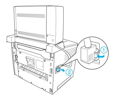
4. Push the buttons located at the bottom of both sides of the main unit, as shown below. Then lift the unit up to remove it from the printer.
