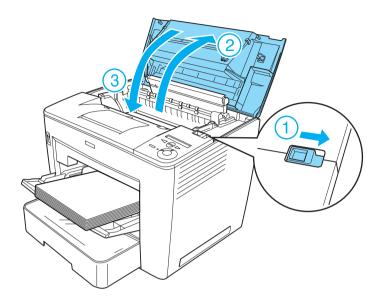
Check the current status of the printer on the LCD panel of the printer's control panel, or from the EPSON Status Monitor 3 utility. If the paper jam error is not yet cleared, check inside the printer. See "Paper jam-inside the printer" on page 284 for instructions.
