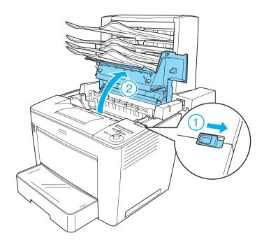
3. Pull out the stopper of the front cover to secure the cover.
