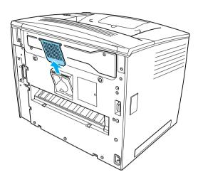
3. Remove the gear cover of the Duplex Unit, as shown below. Use the wrench that comes with the unit to remove the screw.
