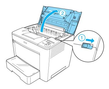
2. Pull out the stopper of the front cover to secure the cover.
