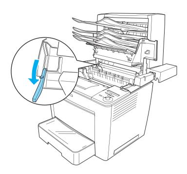
☐ Make sure to push the stopper back to the original position before closing the front cover.
