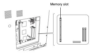
7. Pull the clips on each side of the memory slot outward.
