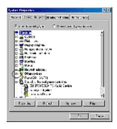
If USB Printer or EPSON EPL-N7000 appears under Other devices, the printer software is not installed correctly. Proceed to step 5.
