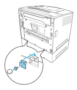
*Note:* Use a coin to tighten the screws.
