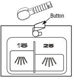
To open the wash cover, press the button and the cover will flip back.
