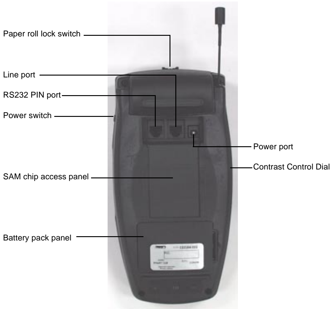
Figure 2-1. ICE 4000 under panel connectors
