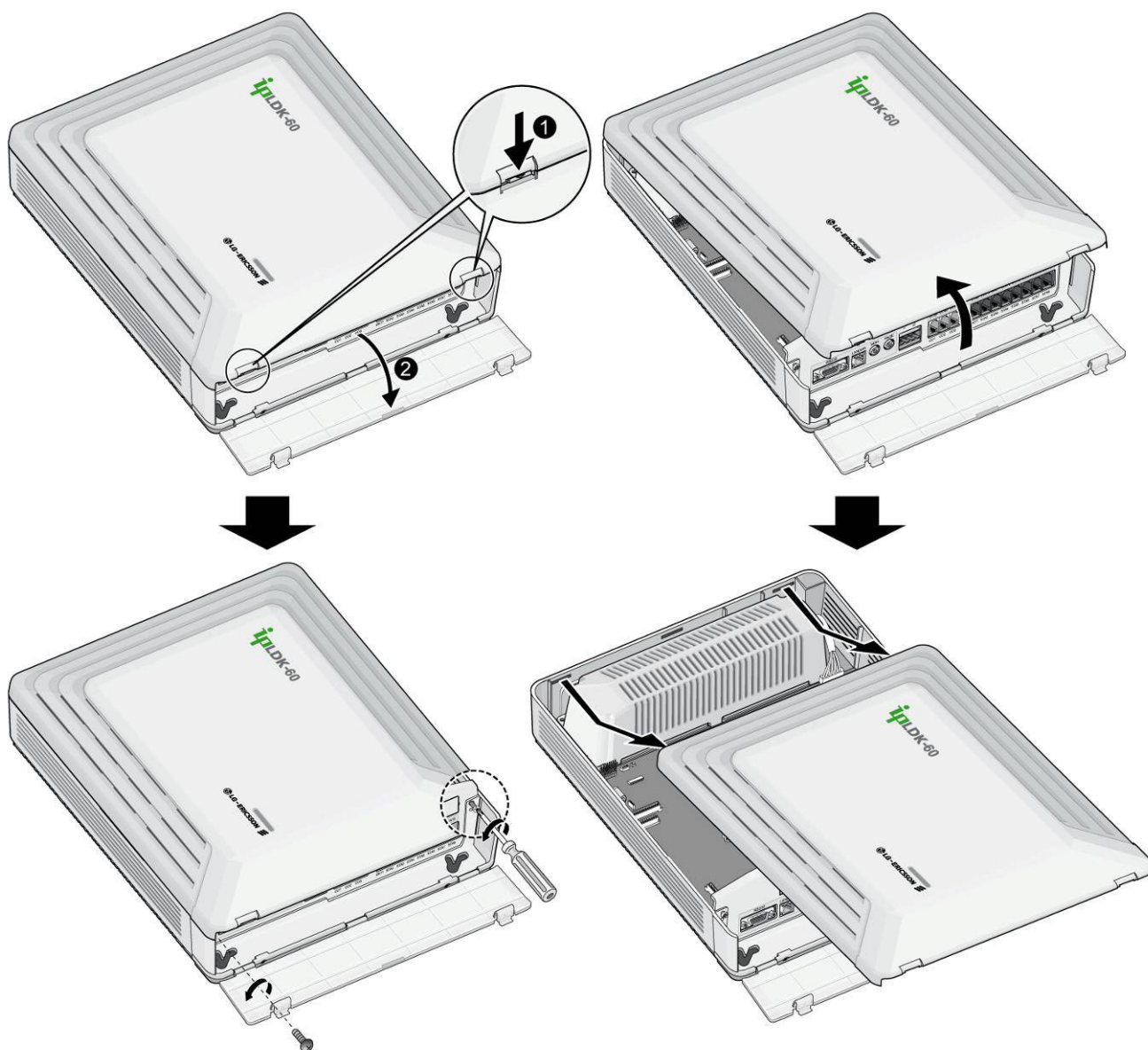
FIGURE 3.2.3.1 OPENING THE FRONT COVER
