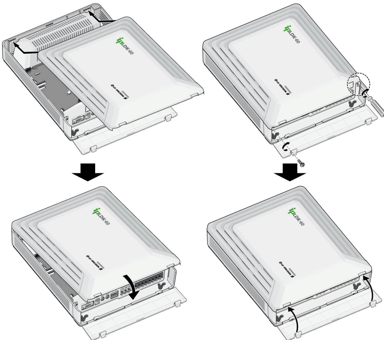
FIGURE 3.2.3.2 CLOSING THE FRONT COVER
