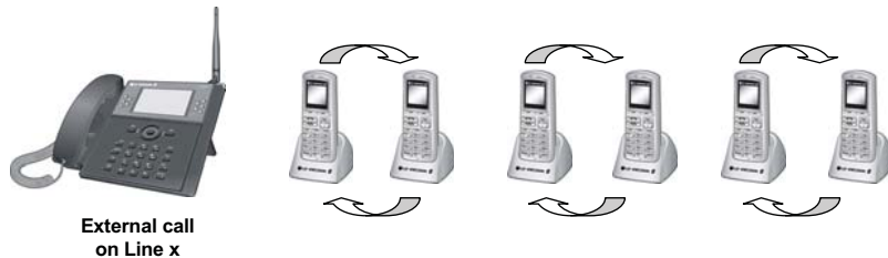
Figure 1.4-3 – Internal Calls Supported
