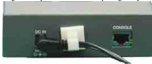
Figure 3-6 Connecting power connector to DWDM-ONT through holder
