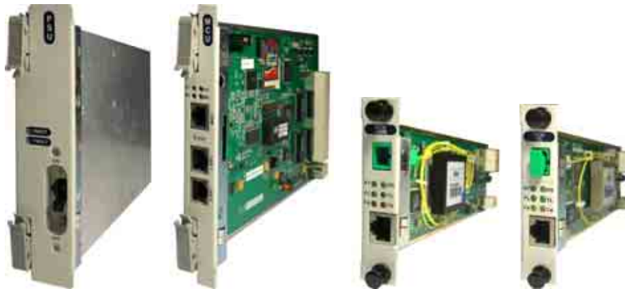
Figure 1-4 PSU, MCU, OCU-100M, and OCU-1G
