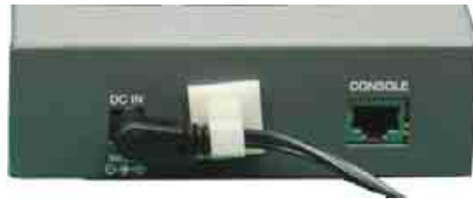
Fig. 3-6 Connecting power connector to DWDM-ONT through holder
