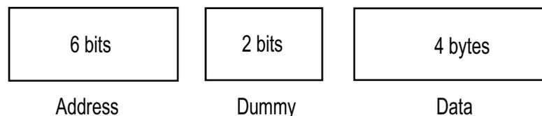
*Figure 5-14 RC Frame Format*
