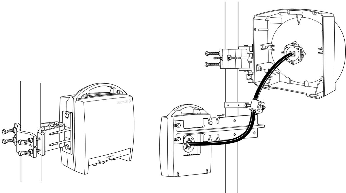
*Figure 8-3 RAU Fitted Directly and Separately to the Antenna*
