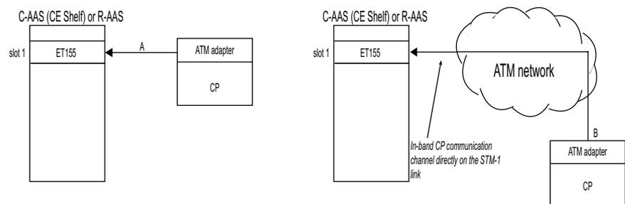
Figure 3–4 CP-SN Connection through ATM Network
