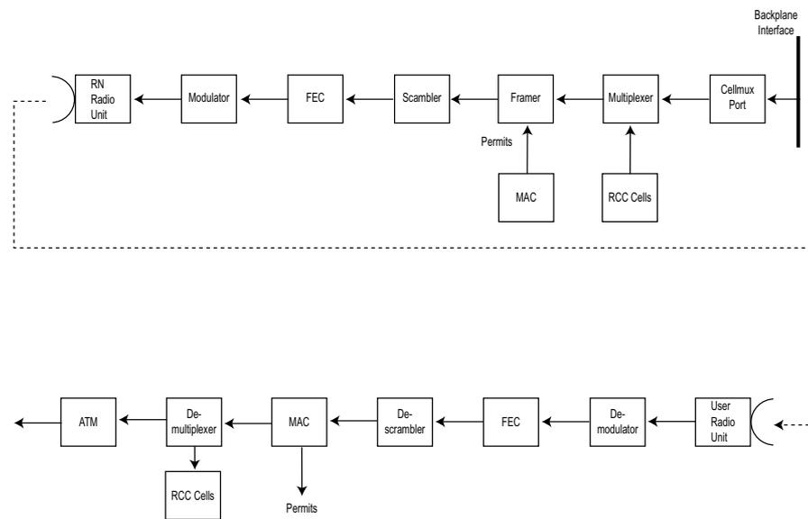
Figure 5-12 Block Diagram for the Downlink Stream
