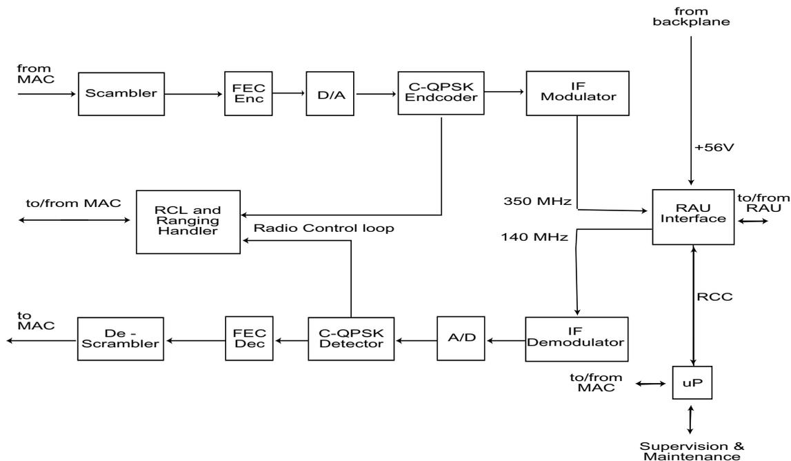
Figure 5-3 Modem Board Functional Block Diagram
