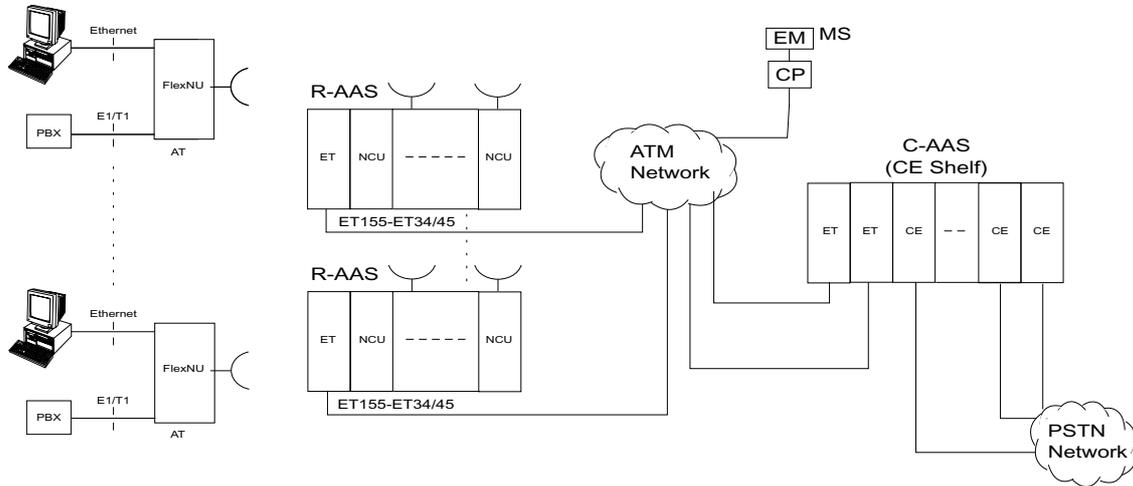
Figure 3-5 Network Example with R-AAS and C-AAS
