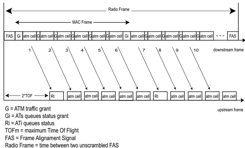
Figure 5-8 Up-Stream and Down-Stream Frames
