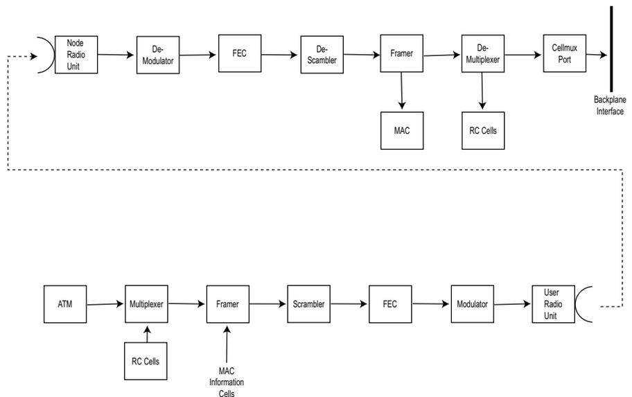
Figure 5-13 Block Diagram for the Uplink Stream
