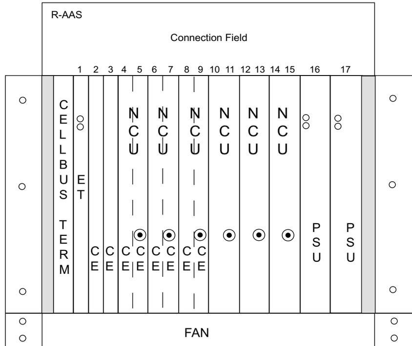
Figure 8-1 R-AAS with Redundant Power
