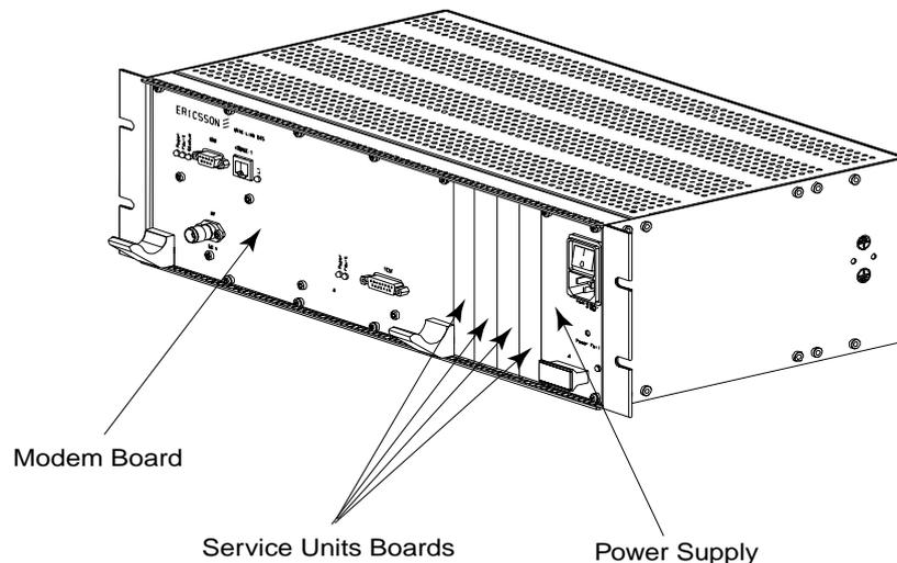
Figure 8-7 The FlexNU Indoor Unit
