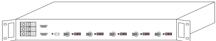
Figure 8-12 5 Outputs PDU Version
