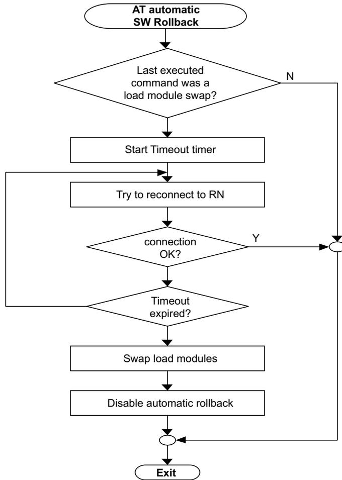
Figure 9-5 Automatic SW Rollback in the AT
