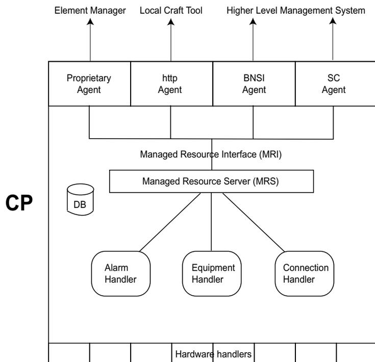
Figure 6-8 CP Software Architecture, Functional View
