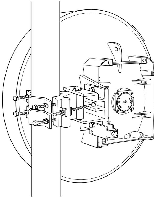
*Figure 8-6 0.60 m Integrated Standard Directive Antenna*
