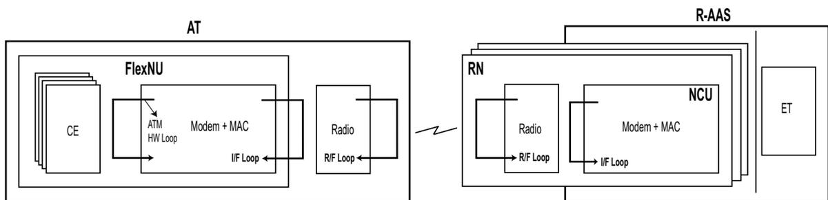
Figure 9-2 RN Near-End Loops and AT Near-End Loops
