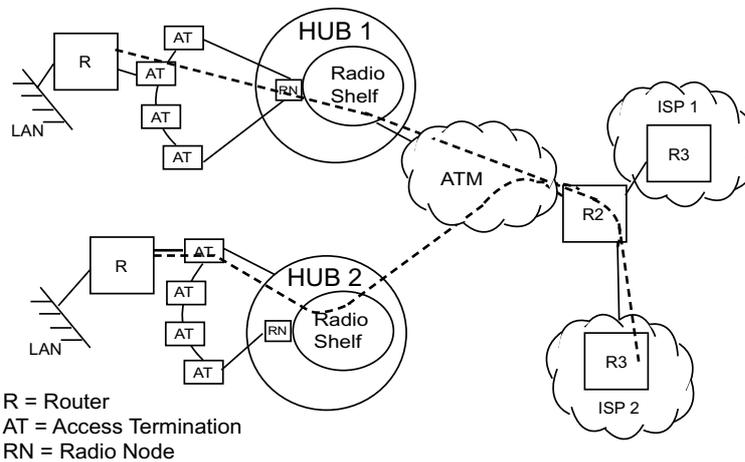
Figure 3-10 System Deployed for Data Traffic and Multiple IP Selection
