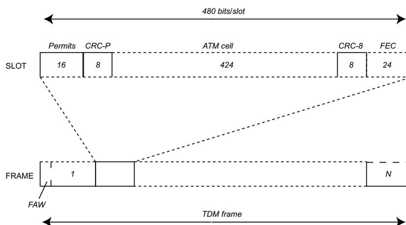
Figure 5-6 Downlink TDM Frame
