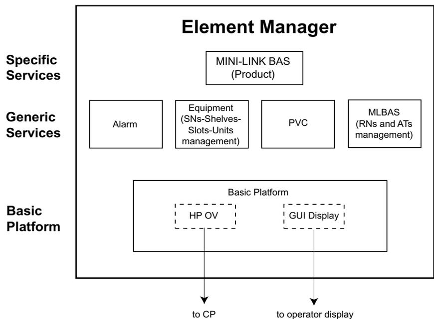
Figure 6-5 EM Software Architecture
