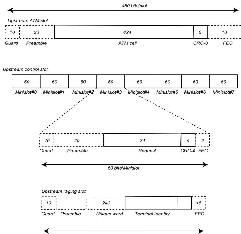
Note: FEC bits are spread over the entire slot
