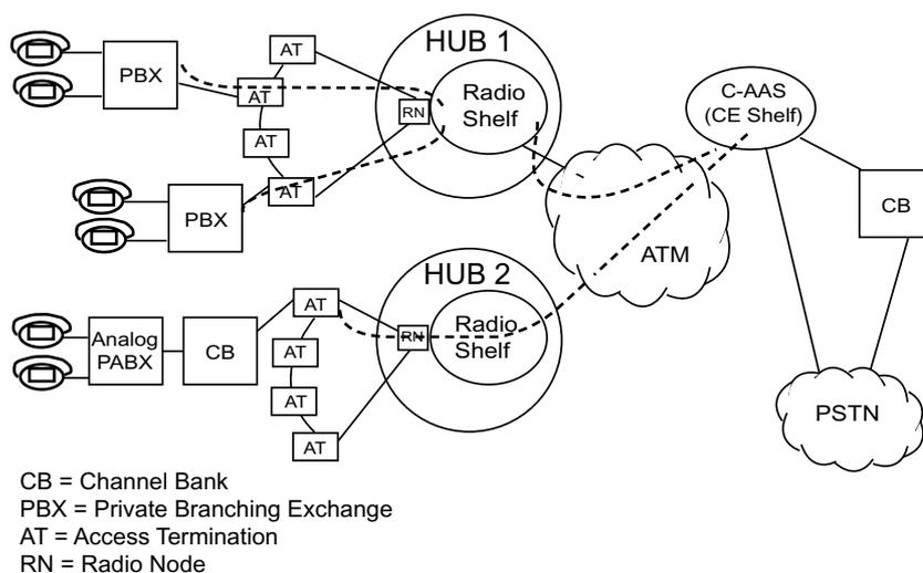
Figure 3-8 System Deployed for Telephony (PBX-PSTN, PBX-PBX)
