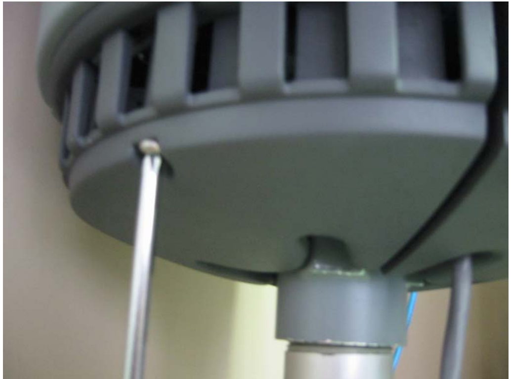
Figure 4: Removing Lower Covers from BelAir200
