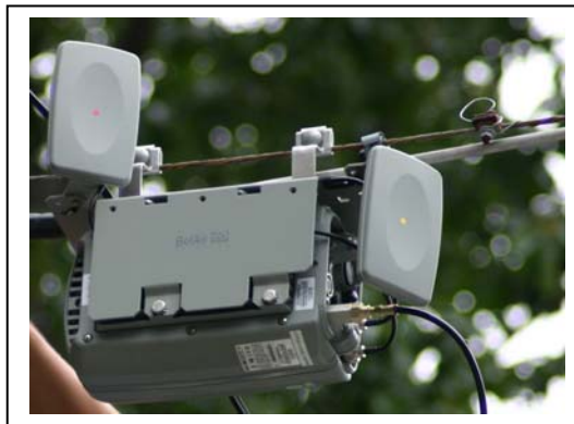
Fig 4. BA100S, strand mount version with B2XH068AA-A module and MTI patch antennas
