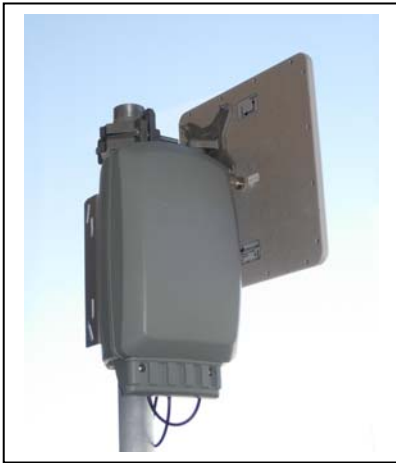
Fig 3. Typical mount of BA100 with B2XH068AA-A module and MTI panel antenna
