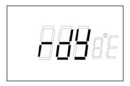
When the logger latches the start command (push button pressed and held for more than one second) the following pattern is displayed for more than 1 second and less than 2, then the logger will either begin logging if the DelayedStart register is set to 0 or enter the delayed start mode if not.
