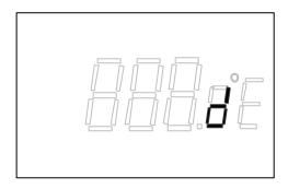
When the logger is in its active logging mode the latest temperature reading is displayed as shown. 'High Alarm 1' and/or 'LOW ALARM 1' will be displayed if the respective alarm is triggered. A low alarm condition has been shown.
