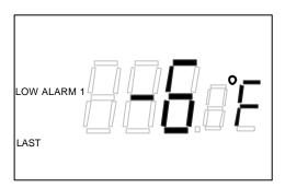
When the logger has finished its program and has stopped logging the following pattern is displayed. If an alarm condition occurred and was latched during logging, it will continue to be displayed. A low alarm condition has been shown.
