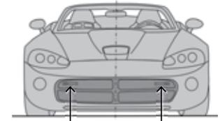
For optimal performance sensors need to be completely unobstructed, not behind a grille, level and facing straight forward (rearward if installing optional rear sensors\*). Make sure that each sensor is parallel with the road (using supplied bubble level).
