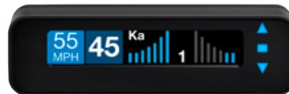
**1** Determine the best location for the Display Module. If installed by a professional, the customer should be consulted. An optimal location is clearly visible from the driver's position and does not take a driver's eyes off the road for more than a moment.
