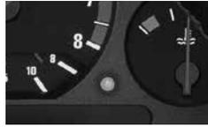
**1** Determine the best location for the Alert Indicator. If installed by a professional, the customer should be consulted. An optimal location is clearly visible from the driver's position and does not take a driver's eyes off the road for more than a moment.
