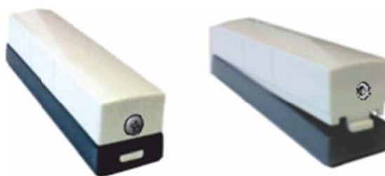
Figure 36: Screwdriver Insertion Point and Top Cover Separation
