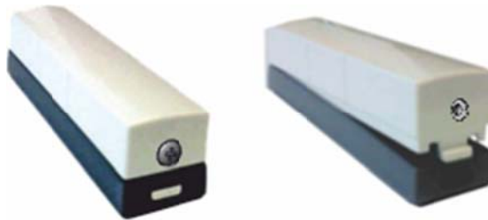
Figure 41: Screwdriver Insertion Point and Top Cover Separation
