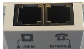
Figure 12: The PSTN Phone Sockets
