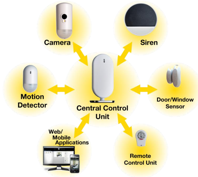
Figure 2: We.R™ Home Area Network Components
